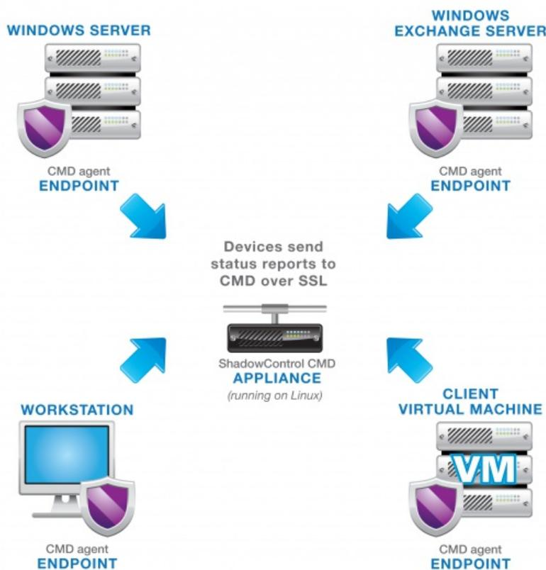
*Each CMD EndPoint reports to the CMD appliance using SSL over Port 443.*
