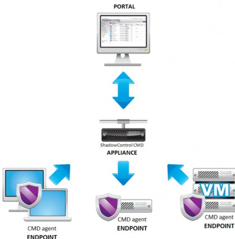
*CMD consists of EndPoints running the CMD agent, an appliance which monitors those Endpoints, and an optional Portal for monitoring multiple appliances.*
